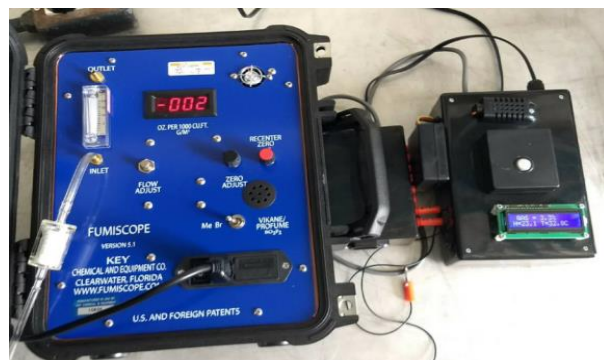
Figure 7 Comparison of Fumiscope Version 5.1 and the developed sensor for measuring methyl bromide in the experiment Source: Photograph by the writer
